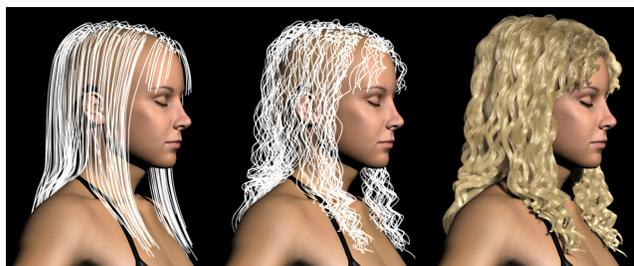
**Figure 9:** (Left) wisp curves generated from a hair mesh, (middle) wisp curves after styling operations, and (right) final hair strands generated from these wisp curves.
