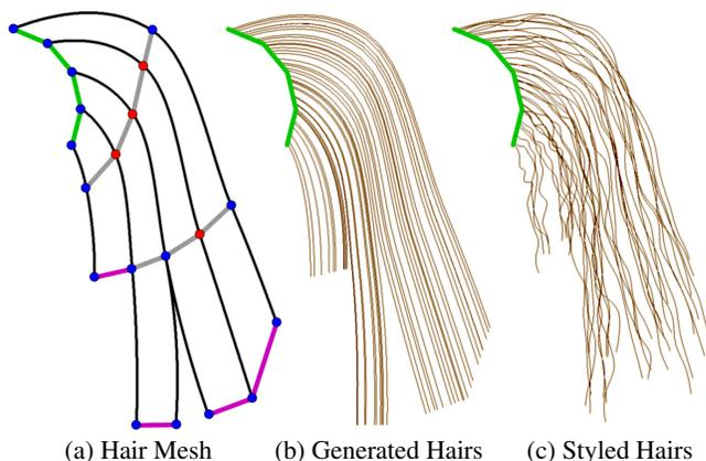
**Figure 2:** (a) 2D representation of a hair mesh, (b) hairs generated from this hair mesh, and (c) hairs after procedural styling operations. The green lines correspond to faces of the root layer, the tip layer is colored purple. Blue hair mesh vertices are external, and red are internal.
