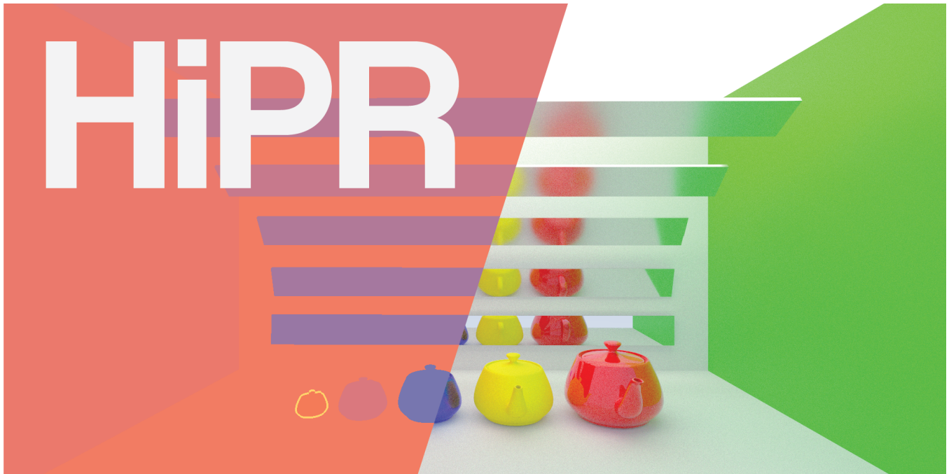
Figure 1: An example scene demonstrating our Hierarchical Progressive Rendering: (left) object id visualization; (right) final rendered image.
