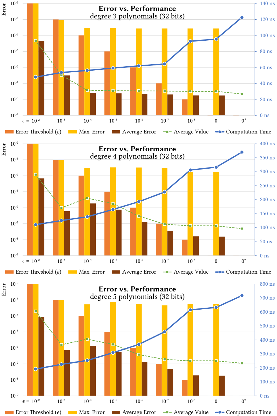
Fig. 4. The error and computation times for different error threshold \epsilon parameters for polynomials of degrees 3, 4, and 5 with single (32-bit) precision.
