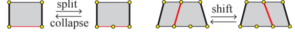
Figure 13: Split/collapse and shift are low-level operations on course and wale edges, respectively.
