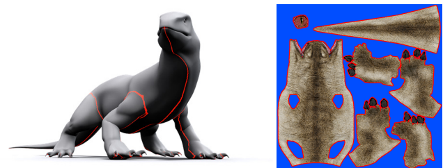
Figure 2: An example character model and its 2D texture layout. The red curves on the model and the texture indicate the seams.
