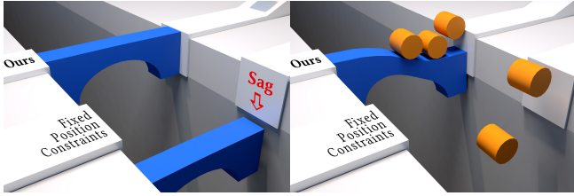
Fig. 5. A soft bridge using our initialization and fixed position constraints. In the latter case, contacts are treated as static and friction is not handled. Our initialization is able to correctly solve for friction and wedge itself between the two cliffs and (left) maintain the initial state until (right) the barrels overwhelm the bridge’s friction. Initializing using fixed position constraints, on the other hand, causes the soft bridge to slide down as soon as the simulation begins.
